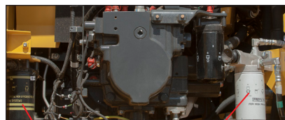
Fuel filter Fuel pre-filter (with water separator)
