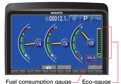
Fuel consumption gauge Eco-gauge
