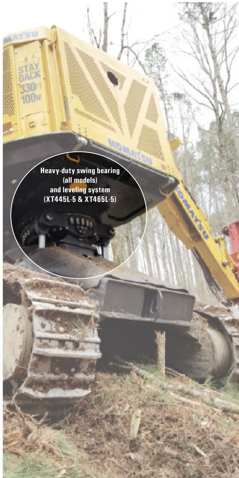
Heavy-duty 4-way leveling system (XT445L-5/XT465L-5)
