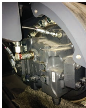
Closed loop track drive
