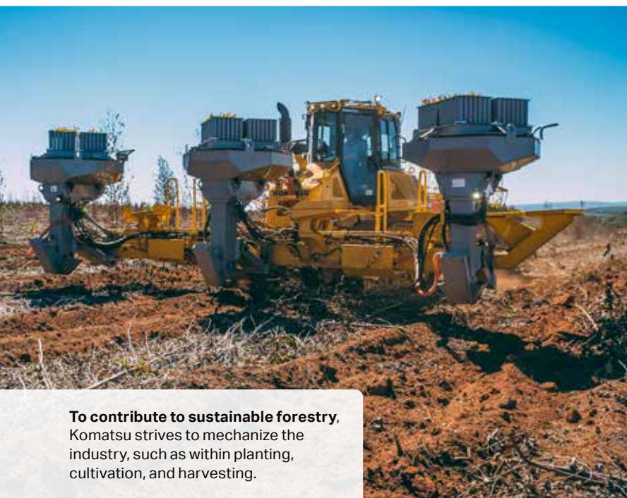
The new planters have transformed the planting process from manual labor performed under the scorching sun to mechanized work in which 900 trees can be planted in an hour, all with exceptional speed and precision.
