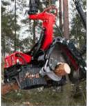
The boom is equipped with a special adapter to increase its outreach. Four special hydraulic pipes are fixed with bolts in the lower part of the excavator's arm and equipped with a protective bracket reducing risk of damage. Lubrication points are transferred to easily accessible location facilitating maintenance.
