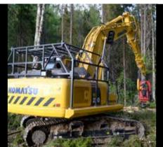
Solid and welldesigned protection of the engine hood and compartments reduces risk of damage and penetration of chips, leaves, and waste from air intakes to the engine compartment, which is an additional fire safety precaution measure.
