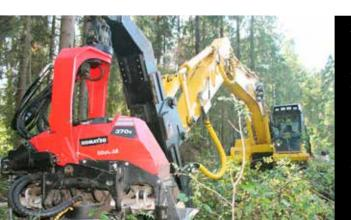
The bucket boom offers additional functionality, i.e. the operator is able to raise the machine, pull out stumps, and conveniently stow the unit for transport, in addition.
