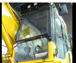
The front window is made of safety polycarbonate glass 19 mm thick to protect the operator against chain break or other mechanical impacts.
