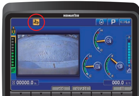
Soot level indicator
