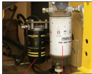
Fuel filter Fuel pre-filter (with water separator)
