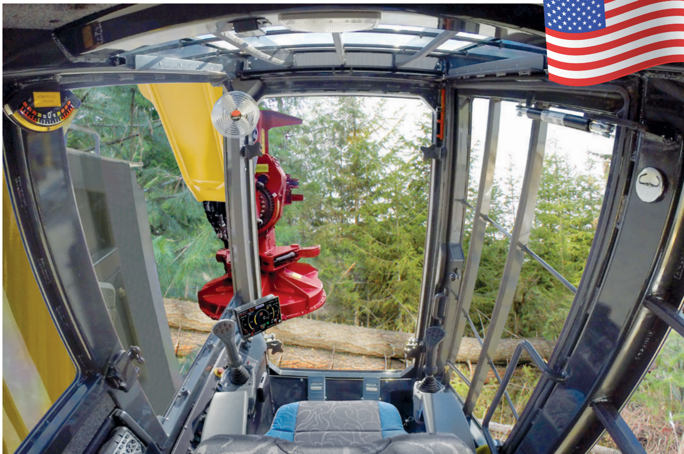
Superior working visibility through all windows and skylight; no window bars on front or boomside windows.
