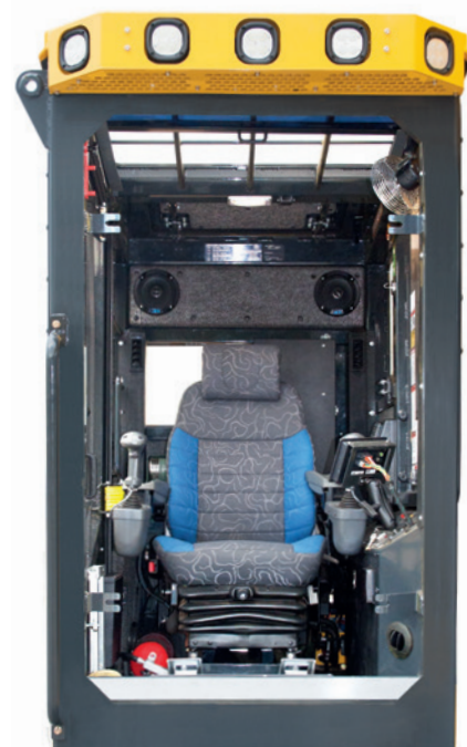
10% larger floor-to-ceiling front window with no footwell or light box obstructions.
