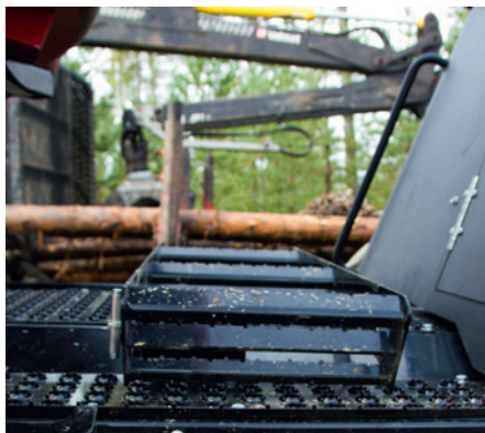
Movable ladder with position sensor.
