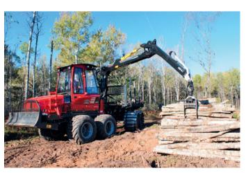
Larry Poquette operating the new Komatsu 855.1 forwarder equipped with the Comfort Ride hydraulic cab suspension system.
