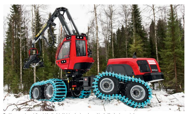
Double suspension entails a rigid articulated joint and swing axle combined with a bogie mounted on the swing axle. Provides maximum mobility and comfort on steep inclines and soft ground.
