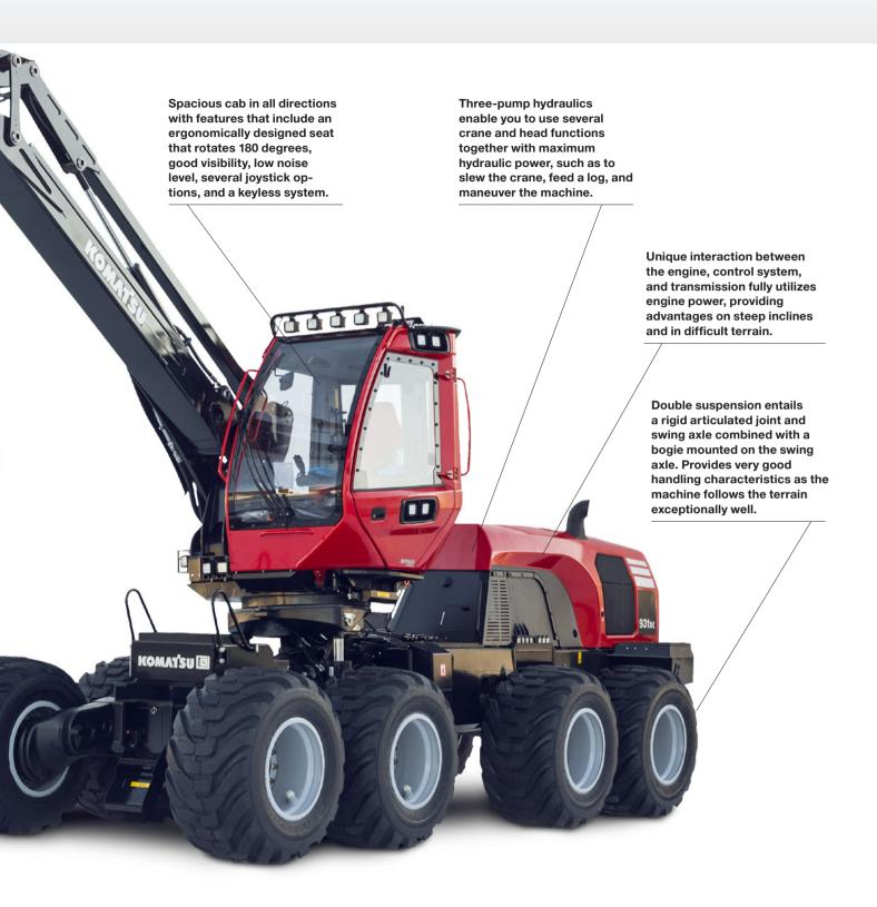
One advantage of an additional pair of wheels is even better stability. Stability at all times is essential if the operator is to be able to maintain productivity regardless of the terrain. The Komatsu 931XC has a unique solution compared to other eight-wheeled harvesters.
