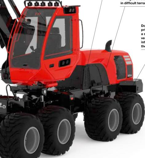
operator environment is unique in several other ways. Large cab volume, good visibility in all directions, smart display placement, and a remote control/key for controlling the main power and cab heater. Underfloor heating, effective lighting, and three joystick options (including EME) to choose between make life in the cab comfortable. You can also choose to add Autolev Advanced cab suspension, which makes for near-perfect cab comfort.
