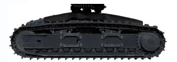
Closed loop track drive with dedicated pumps allows simultaneous multi-functioning of travel, swing, boom and tool without compromising power between work and travel functions.
